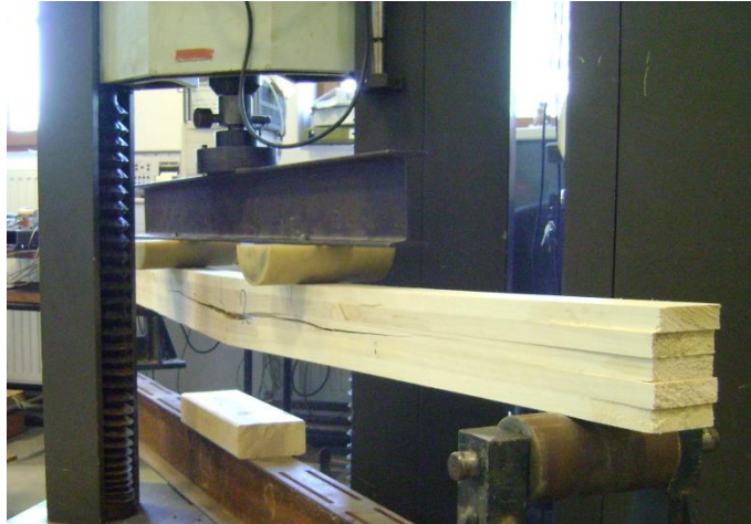
Figure 11: Bending test of a poplar glulam prototype
