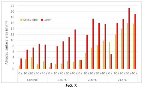
Changes in the abraded (water jet) surface as a result of wood species and heat treatment temperature
