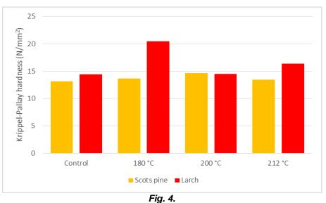
Changes in the surface hardness (side) as a result of heat treatment
