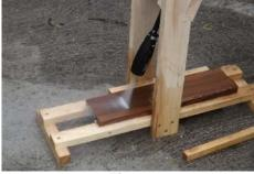
Fig. 1. Sample set of the water jet abrasion
