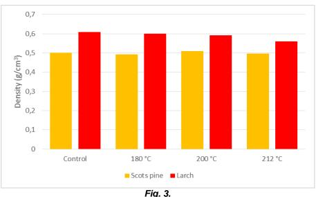
Airdry density of heat treated and control samples
