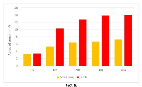
Effect of time of the high pressure water jet on the abraded surface area (0 sec. means surface roughness).
