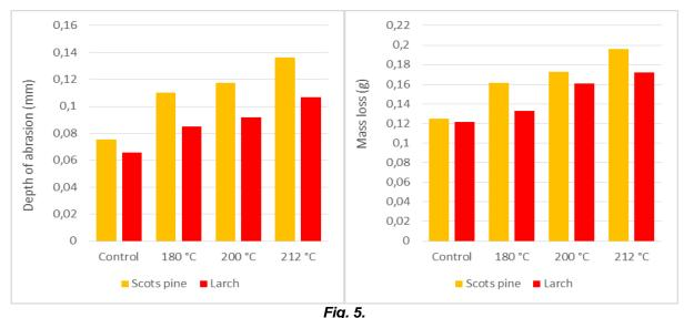
Changes in the mean Taber abrasion for 100 turns as a result of heat treatment
