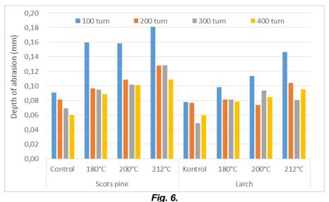
Changes in the Taber abrasion per each 100 turns during abrasion as a result of heat treatment
