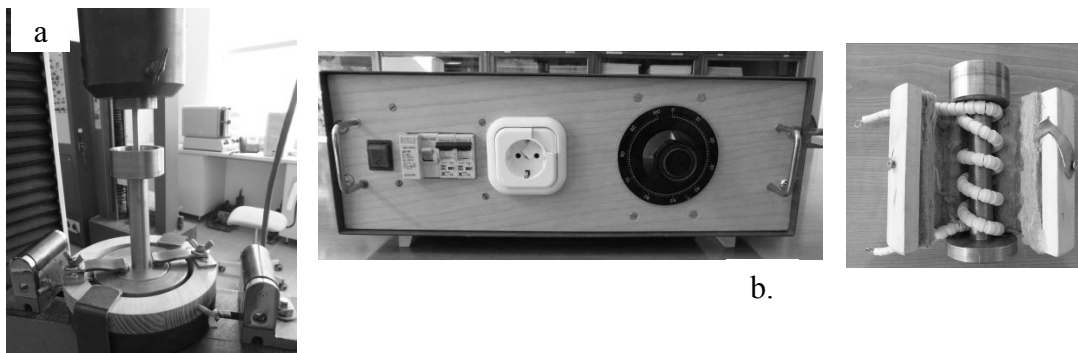
Fig. 1 Punch and the temperature control and measurement system
