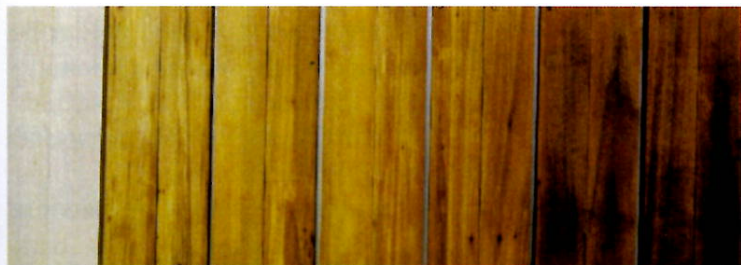
Fig. 2. Colour change of poplar wood due to different heat treatment schedules in linseed oil
