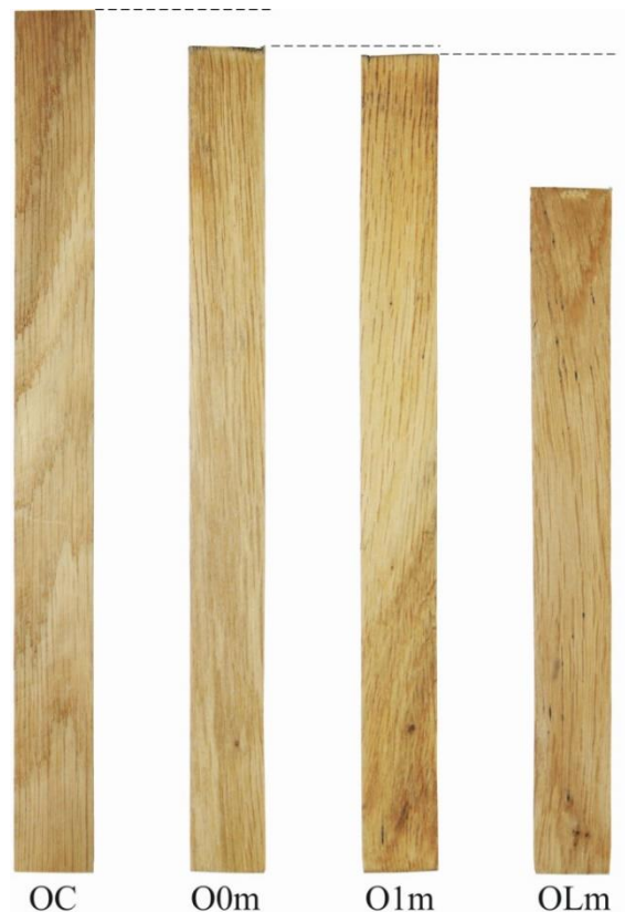
Figure 1. Shortening of samples from different treatments. Abbreviations: OC – control sample; O0m – longitudinally compressed sample; O1m – longitudinally compressed sample relaxed for 1 minute; OLm – longitudinally compressed sample relaxed for 18 hours.
