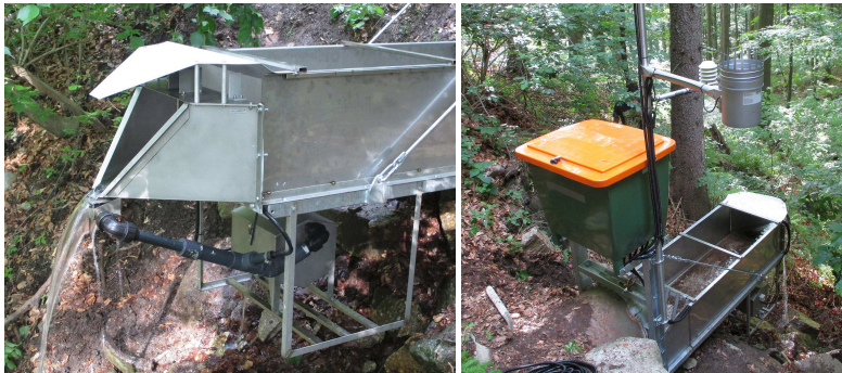
Figure 6: H-flume type runoff gauge at Rosalia basin (tributary Mittereckgraben)
