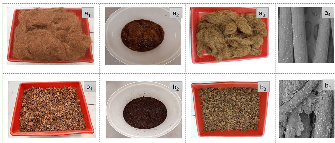
Figure 1. Photographs of coir fibers: (a 1 and b 1 ) before pretreatment; (a 2 and b 2 ) coir fibers in alkaline solutions; (a 3 and b 3 ) coir fibers after treatment; (a 4 and b 4 ) morphological views of coir fibers.
