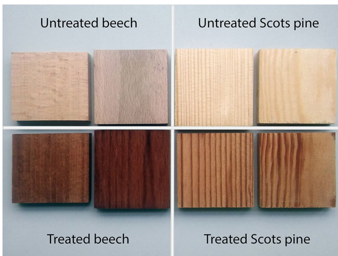
Fig. 13 Colour change of beech (left) and Scots pine (right) wood material as a result of different silica aerogel treatments
