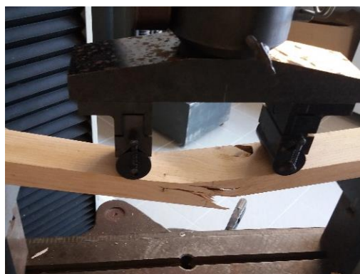
Figure 2: Static bending test according to EN 408:2010 + A1 (2012)
