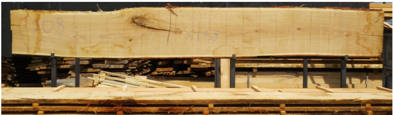
Figure 1: Sample No. 208 used for visual classification, with several typical wood defects
