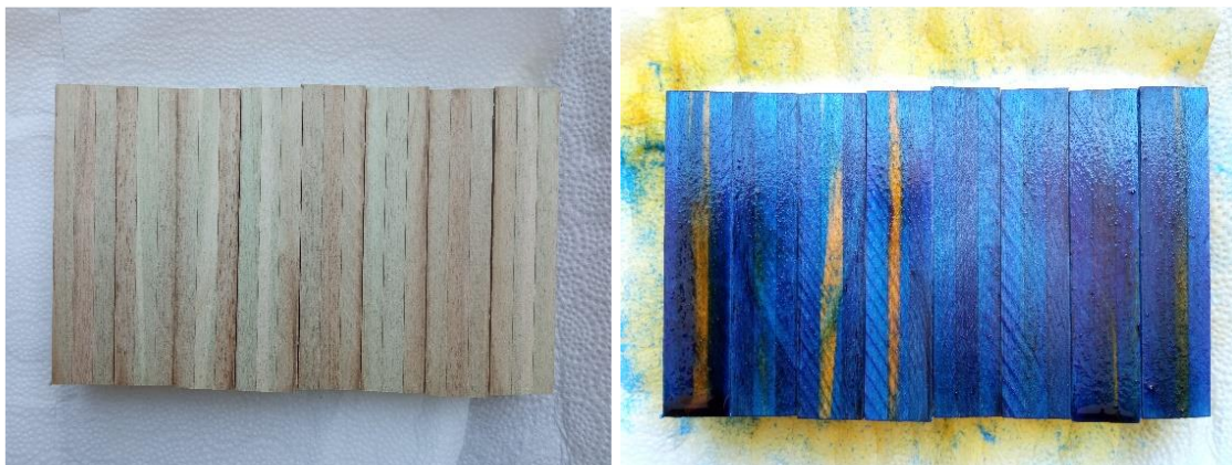
Figure 4: Longitudinally-cut glued-laminated specimens before (left) and immediately after (right) treatment with reagent
