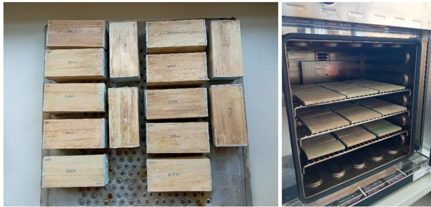
Figure 3: Dried glued specimens (left) and reference lamellas in dryer (right)
