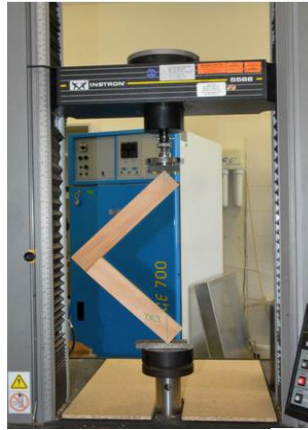
Figure 4: Display of test samples on the test machine; corner joint sample with tensile test
