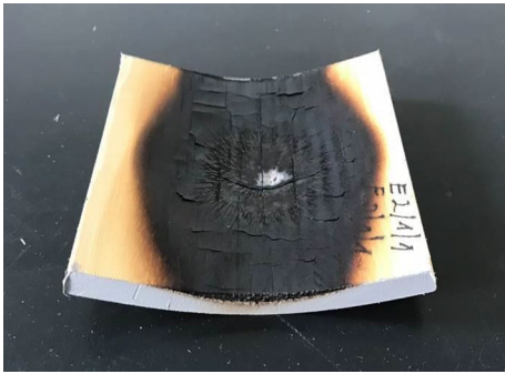
Fig. 7 Concave deformation of Scots pine
