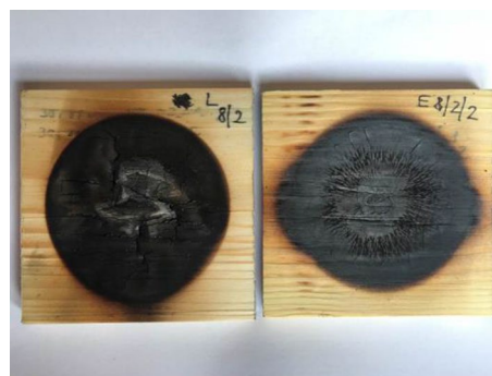
Fig. 6 Visible cracking of the test samples
