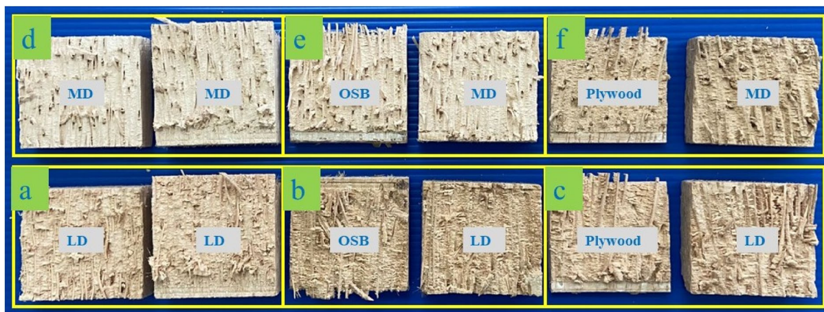
Fig. 4 Shear plane surface of the specimen after block shear test (a) low density oil palm wood bonded with low density oil palm wood, (b) low density oil palm wood bonded with OSB, (c) low density oil palm wood bonded with plywood, (d) medium density oil palm wood bonded with medium density oil palm wood, (e) medium density oil palm wood bonded with OSB and (f) medium density oil palm wood bonded with plywood
