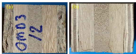
Fig. 10 Representatives of failure modes observed in the test specimen after compression test (a) OSB face sandwich panel with low density core, (b) plywood face sandwich panel with low density core
