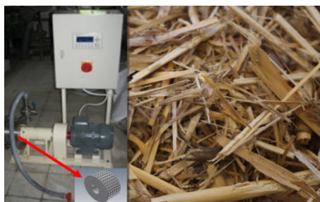
Figure 1 The hydrodynamic cavitation device (left) and Miscanthus raw material (right)
