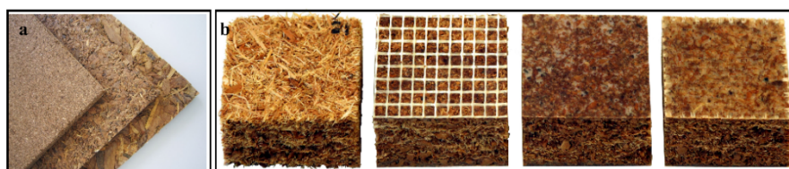
Figure 2 Black locust bark panels (a) and overlaid GFRP panels (b)
