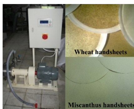
Figure 3 Hydrodynamic cavitation device and agro-waste paper handsheets
