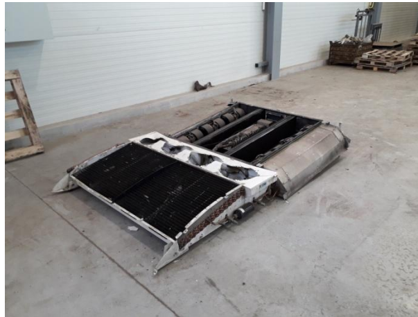
Figure 4. Air conditioner of Ikarus 395
