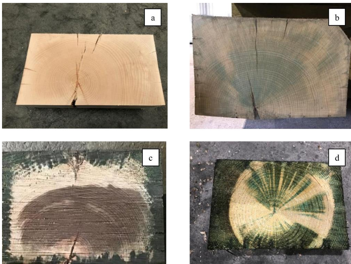
Figure 3: Cross-section of beech sleeper before saturation (a), Cross-section of fully saturated beech sleeper with water-based preservative (b), Image of saturated area after second saturation with SleeperProtect (beech, dark green area) (c), Image of saturated area after second saturation with SleeperProtect (Scots pine, dark green area) (d)
