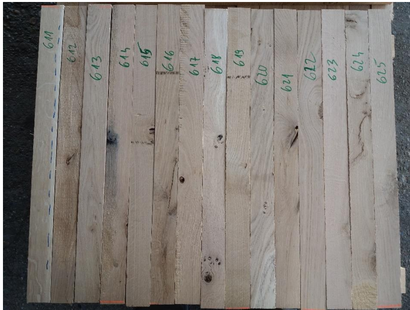
Figure 1: Typical wood failures in the lamellae used for the specimens
