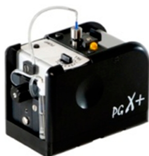
Figure 1. The PG-X goniometer used for the measurements.
