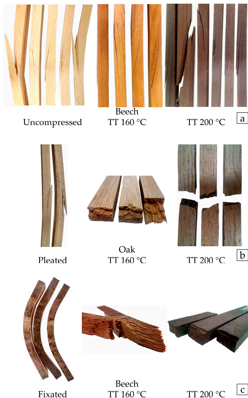
Figure 3. Typical fracture images of (a) not compressed; (b) pleated; (c) fixated samples with and without thermal treatment. Abbreviations: Pleated—steamed and compressed along the grain by 20%; Fixated—pleated, then kept compressed for 5 h; TT 160 °C—thermally treated at 160 °C; TT 200 °C—thermally treated at 200 °C.
