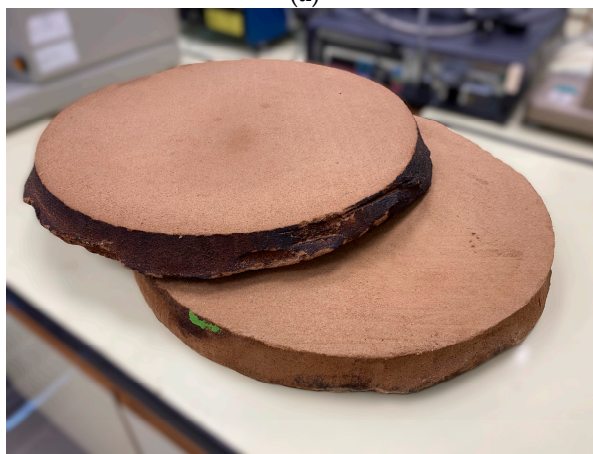
Figure 1. (a) Milled bark before the defibration process for insulation board production. (b) Example of the fabricated panels after sanding (upper panel made of Robinia pseudoacacia (Black locust) bark fibers, lower; lower panel made of Tilia spp. (Lime)).
