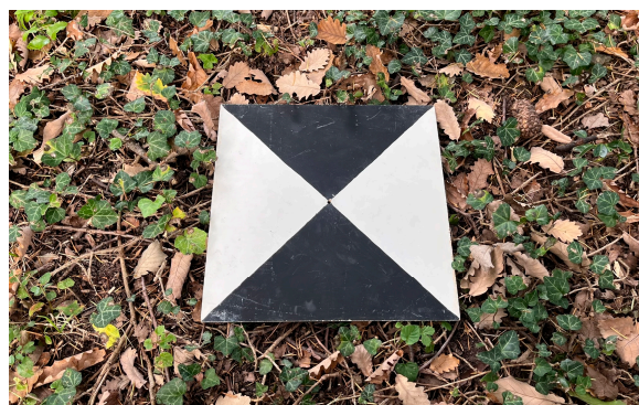
Figure 5. Example of a ground control point used in the survey.
