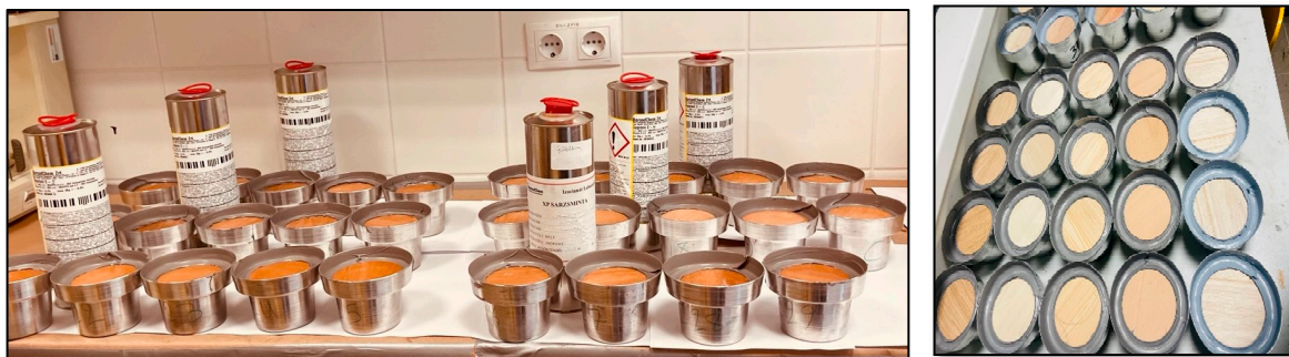
Figure 2. (Left) side: samples prepared according to ISO 12572 and the 5 custom made polyol formulations with different molecular weights and the custom made adhesive; (right) side: cups with the Smaragdfa disks coated with the listed polymers.
