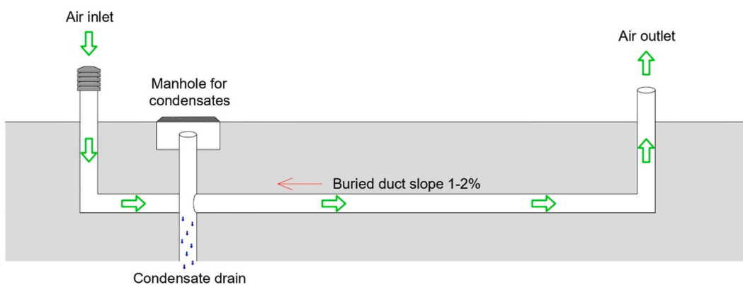
Fig. 3. Scheme of the EAHE drainage system.
