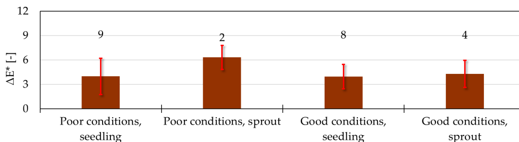
Figure 5. Average total color differences ( \Delta E^* ) of the boards, grouped by growing site type. The difference between the average color components of each specimen and the entire sample set averages used in this study was calculated. The diagram shows the averages of the \Delta E^* values for the specimens belonging to each site type. The average \Delta E^* values shown in the diagram were obtained by averaging the calculated \Delta E^* values by growing site type. Standard deviation is shown by red bars, while the numbers above the bars denote the sample size included in the statistical evaluation.
