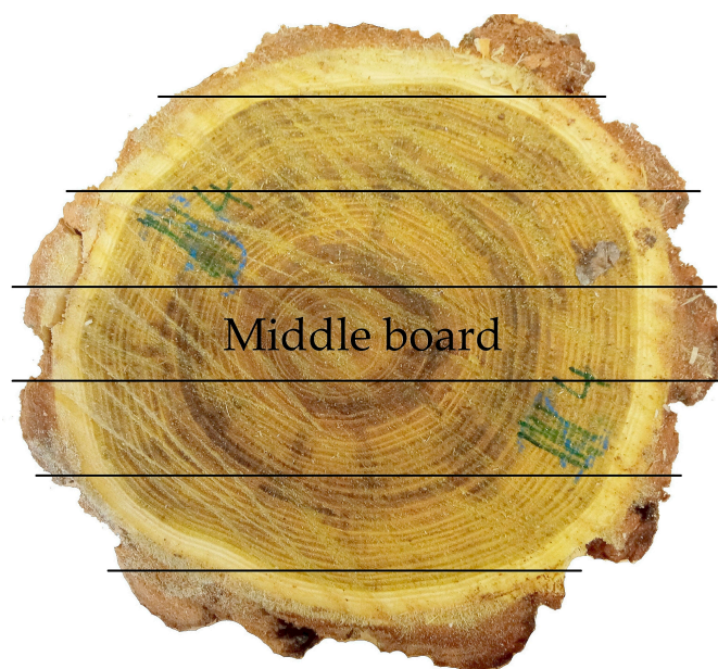
Figure 2. The location of the board from the central heartwood (middle board) specimens used within the log.
