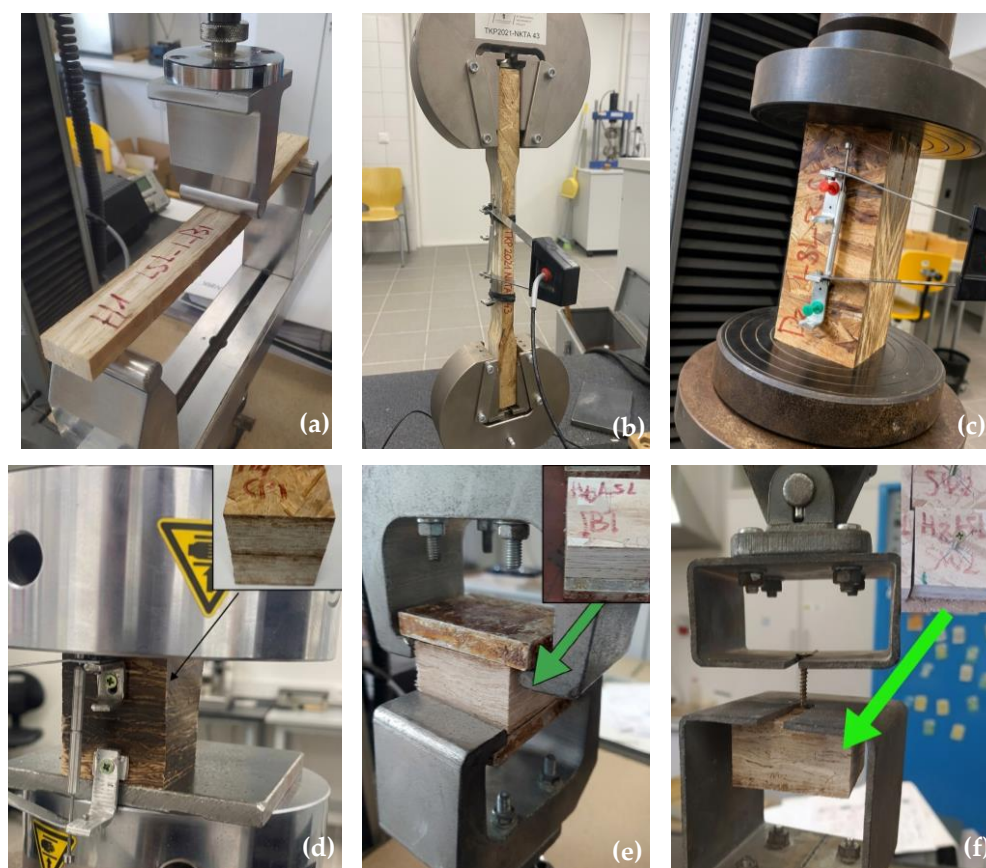
Figure 4. Mechanical tests of OSL panels: (a) bending; (b) tension; (c) in-plane compression; (d) flat-wise compression; (e) internal bond strength; (f) screw withdrawal resistance.
