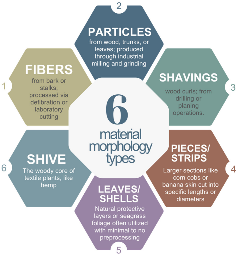
Figure 4. Structural forms and morphology of plant-based materials used in bio-based thermal insulation materials.
