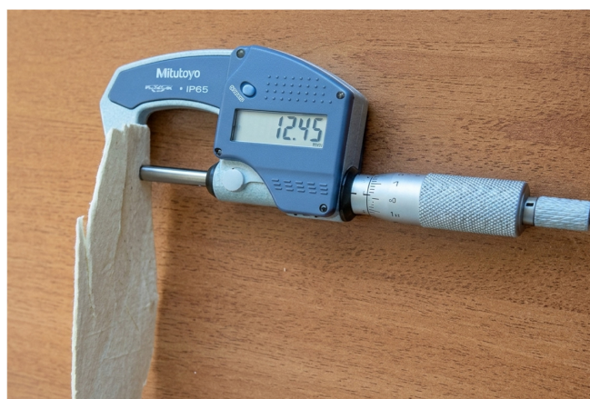
Figure 2. Digital micrometer used to determine strand thickness at five points (S1–S5) along the centerline.
