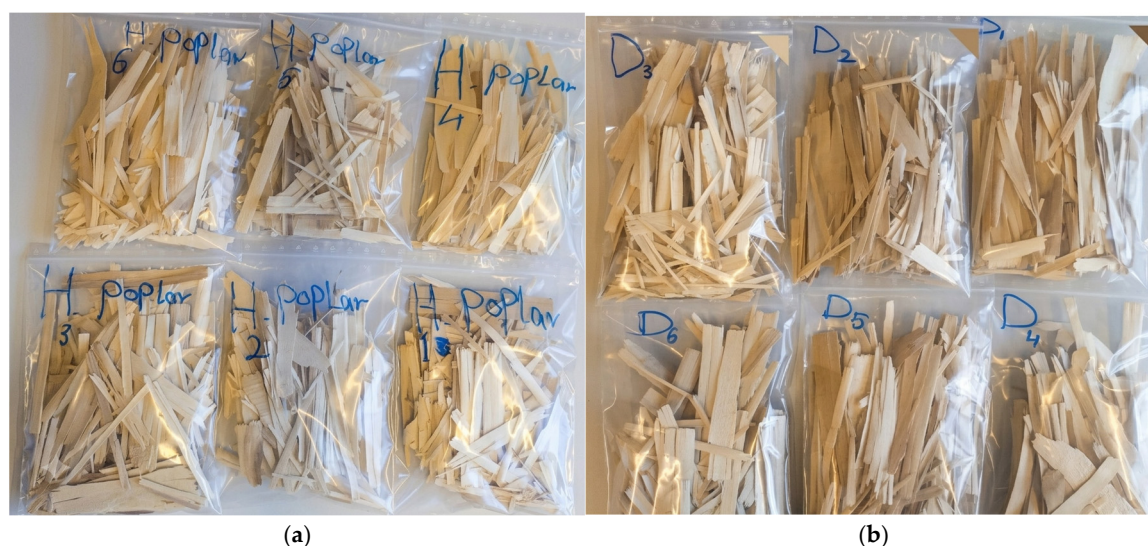
Figure 1. Hybrid (a) and indigenous (b) poplar strands used in morphological measurements.
