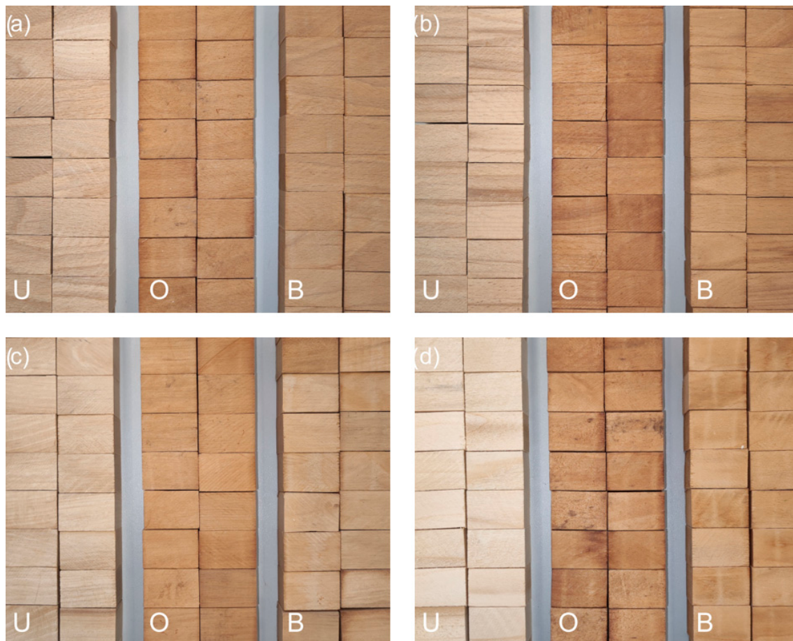
Figure 2. Photographs of samples used for color testing. The images show specimens of beech (a), beech with false heartwood (b), hornbeam (c), and poplar (d). In each image, the specimens are arranged from left to right as follows: untreated samples (U), samples impregnated with oak bark extract and subsequently fumed (O), and samples impregnated with beech bark extract and subsequently fumed (B).
