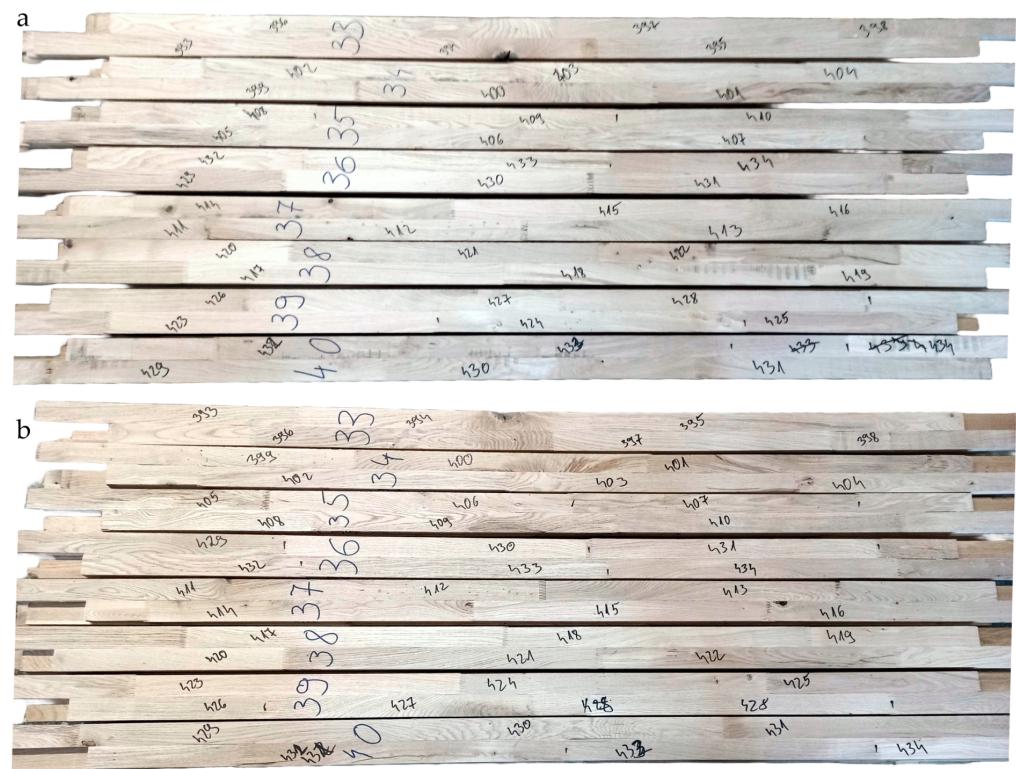
Figure 1. The lamellae were glued together to form elements. Images (a,b) show the two sides of some elements. Typical wood defects can be seen such as pin knots, sound knots extending through the full cross-section, decayed knots, slope of grain, cracks, and sapwood.
