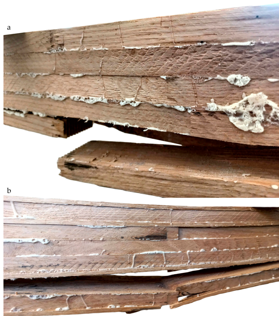
Figure 4. Typical bending test failure of GLTs made exclusively of oak lamellae (a) and of oak lamellae reinforced with veneer layers (b).
