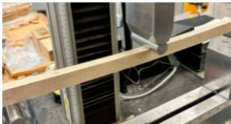
Figure 3. Edgewise bending test of an I-214 poplar test piece with PF adhesive.
